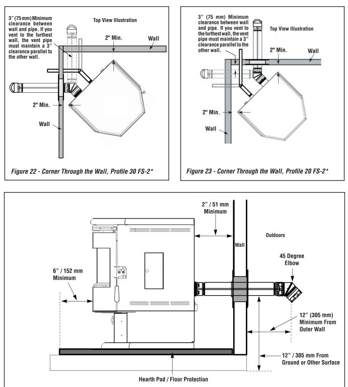
Figure 24 - Parallel Through the Wall, Profile 20 FS and Profile 30 FS
